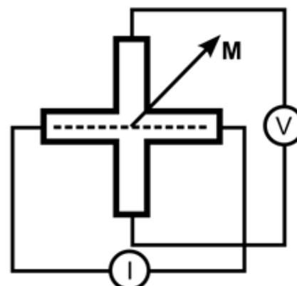
Fig. 5: Illustration of the micro-Hall sensor design.
