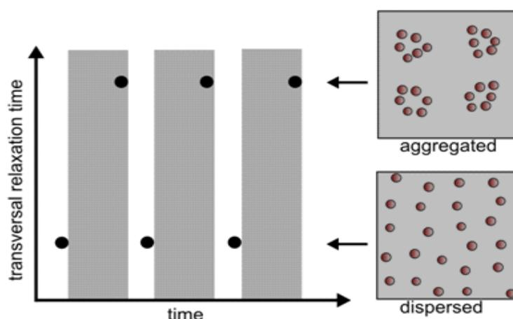
Fig. 3: Principle of magnetic relaxation switches. The grey area in the graph indicates that a homogenous magnetic field is turned on.
